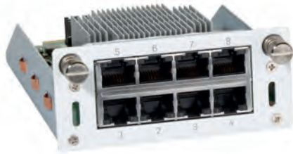
8 port GE copper FleXi Port module
